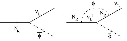
Self energy diagram interfering with tree level diagram. This is similar to CP violation in  $K - \bar{K}$  oscillation (indirect CP violation entering in the mass matrix). [M. Flanz, E.A. Paschos and US, PLB 95]
