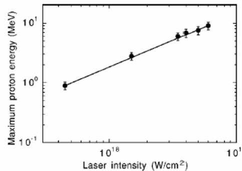
FIG. 3. Maximum proton energy in the forward direction as a function of laser intensity for  $6\ \mu\text{m}$  Mylar foil.
