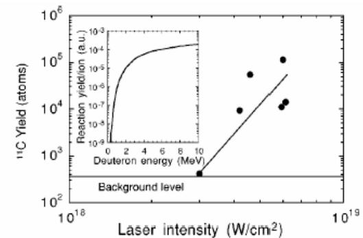
FIG. 4. Experimental yield of  $^{11}\text{C}$  vs the laser intensity for the  $^{10}\text{B}(d,n)^{11}\text{C}$  reaction. The inset shows calculated yield of  $^{11}\text{C}$  per one deuteron as a function of energy cutoff  $E_{\text{max}}$  for a uniform distribution of deuterons in energy space.
