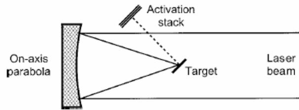
FIG. 1. Schematic experimental layout in the on-axis geometry. Laser beam entering from right-hand side is focused by the parabola (left-hand side) to target surface (middle). Blow-off plasma hits activation sample (top) in the target normal direction.
