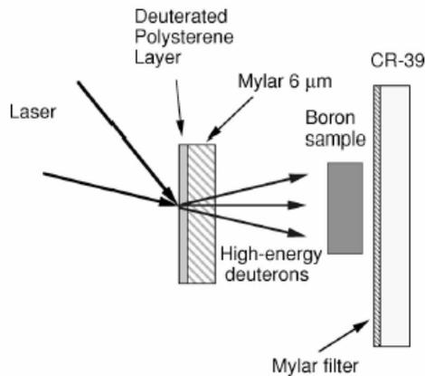
FIG. 2. Schematic diagram of the boron sample activation with high-energy deuterons.
