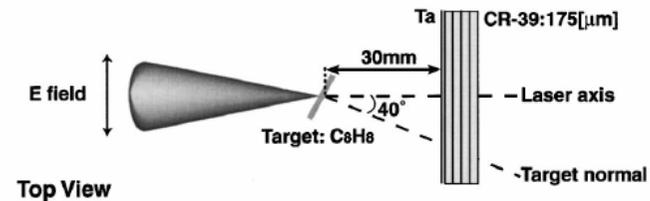
FIG. 1. CH target and CR-39 track detector setup. Target is 3 mm square in size and 5 to 100  $\mu\text{m}$  in thickness. CR-39 film, stack of four layers, covered with Ta foil, is 6 cm in diameter, and is put 3 cm apart from target.
