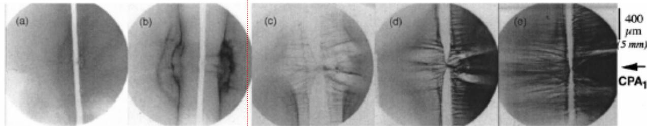
FIG. 3. Proton images of the interaction zone after irradiation with the CPA<sub>1</sub> pulse of a 50 μm Ta wire for different interaction-probing delays: (a) -15 ps; (b) -5 ps; (c) 5 ps; (d) 15 ps; (e) 25 ps. The energy of the protons employed was 6–7 MeV. Here and in the following figures spatial scales for both the target and the image plane (between bracket) are indicated.
