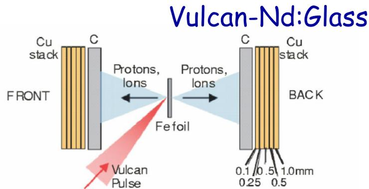
FIG. 1. (Color online) Experimental arrangement used for diagnosing ion acceleration using nuclear activation techniques.
