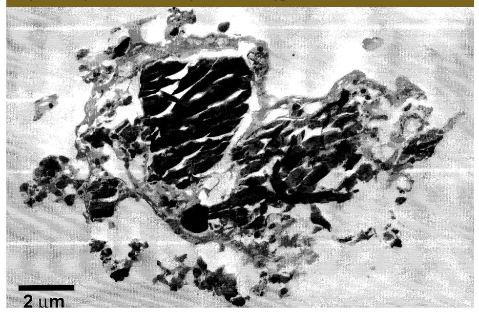
■ Typical dust particle (650 nm size) grown in a plasma processing reactor (SEM image: Garscadden et al. 1994)
