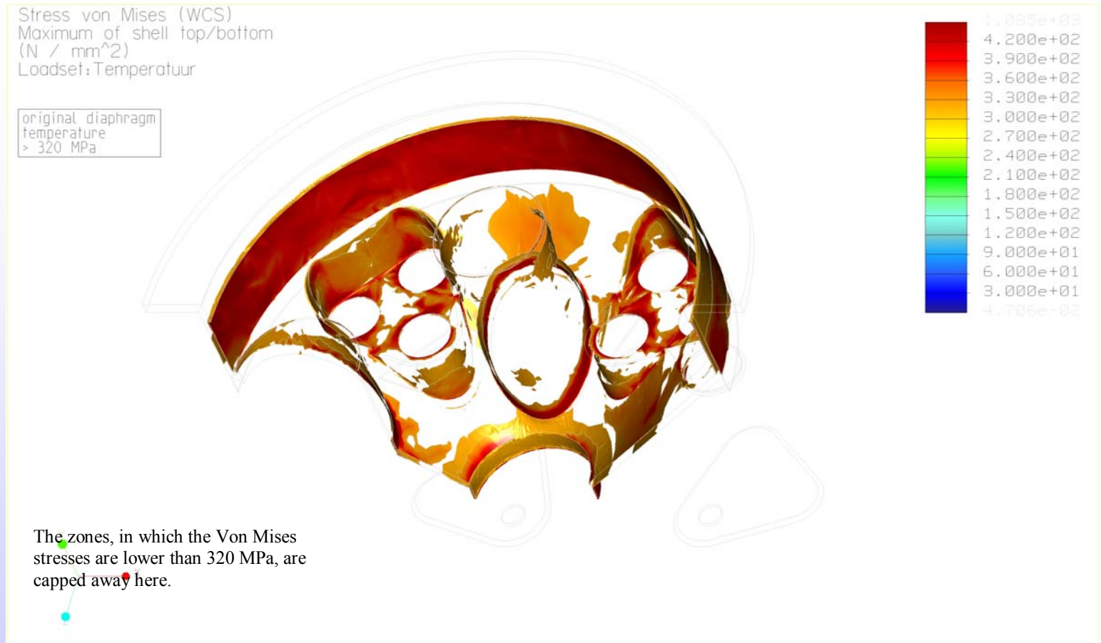
Figure 10. Von Mises stress for thermal load.
