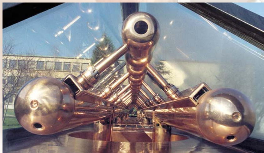
Historical examples: a Wideroe type structure (ALICE heavy ion injector, IPN Orsay)
