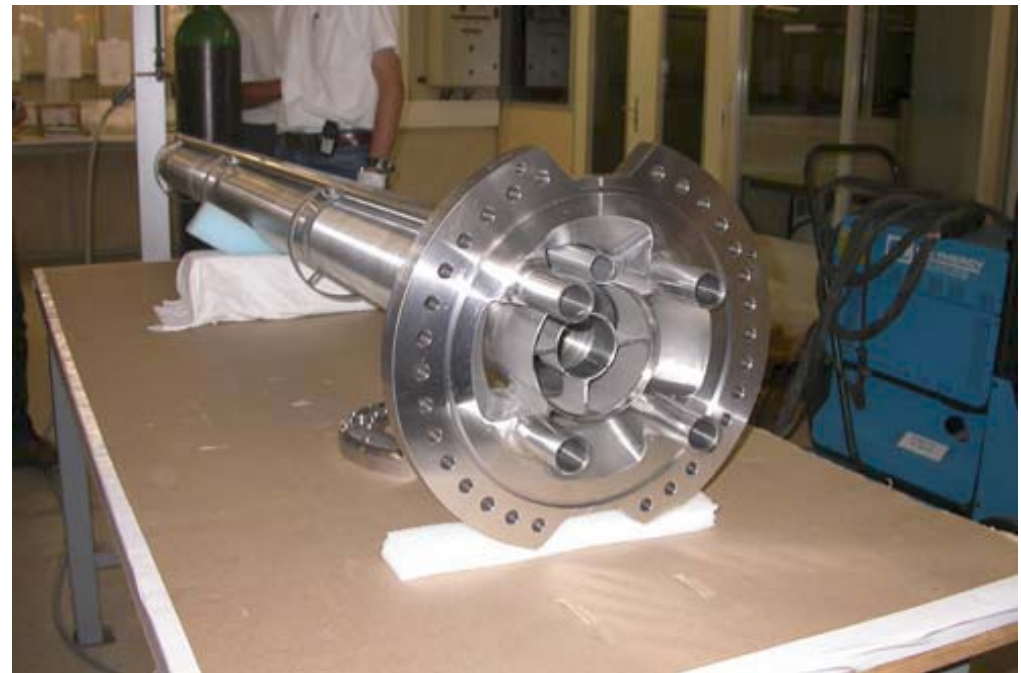
The central flow guide tube
