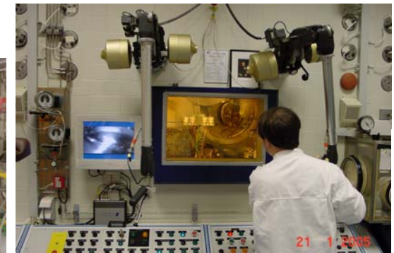
Pilot facility for pyrometallurgical reprocessing
