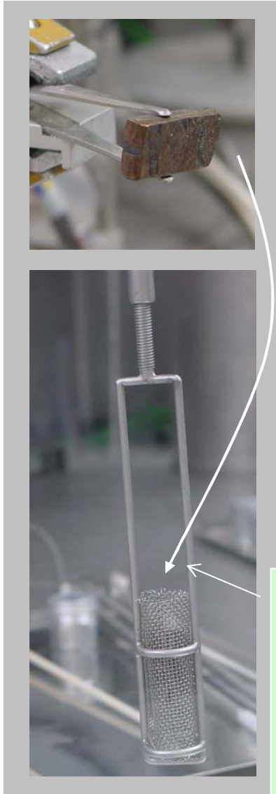
anode basket loaded with Pu/Am metal (45g)
