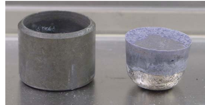
Recovered Cd-Pu/Am ingot and AlN crucible
