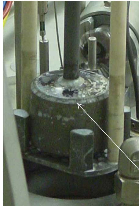
anode basket loaded with Pu/Am metal (45g)
