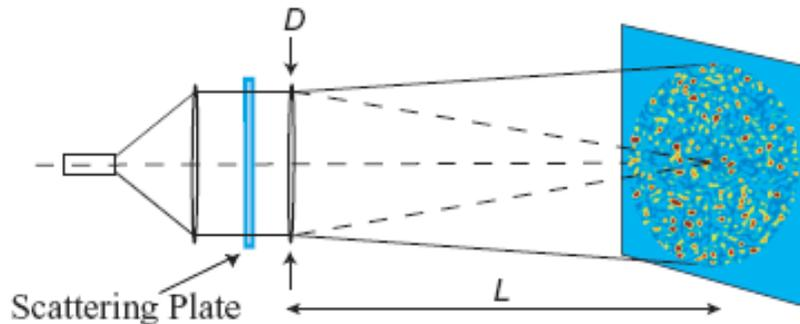
Laser speckle: very well controlled random intensity pattern (Gaussian random process, central limit theorem)
