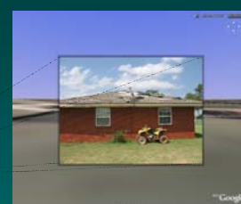
FIG 7: One "enhanced" image, which is placed into Google Earth™ with image three-dimensionally oriented in direction photograph was taken.
