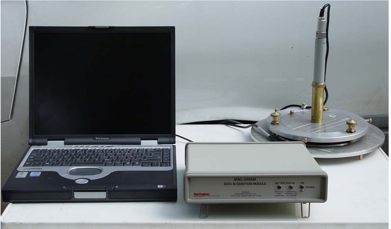
Fig. 8. Recording system MAG-03 DAM (Bartington, England)
