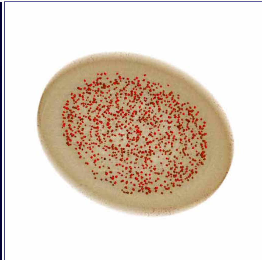
Tomography slice of one layer with CP
