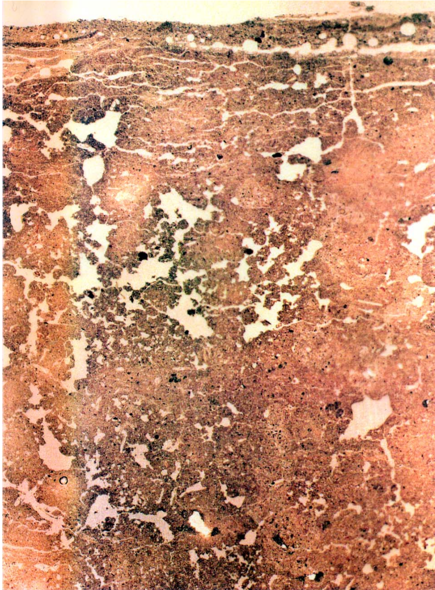
Figure 6 - Macrophotograph of a vertically oriented thin section from undisturbed samples of the surface of conventionally ploughed loam soil. In this case the crust appears thicker than that represented in Figure 5. The porosity is also higher but formed by some "vesicles" and planar pores, some also large, oriented parallel to the soil surface. The continuity in a vertical sense is practically absent. Picture taken under a macro-epidiascope with plain polarised light. Frame length 3 cm.
