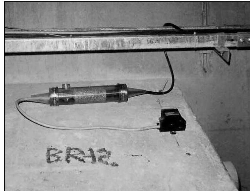
Uniaxial Accelerometer (Horizontal Transverse Acceleration)
