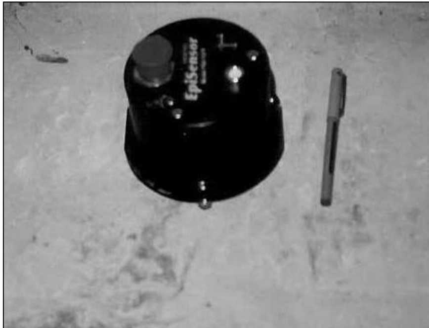
Triaxial Accelerometer (Acceleration in 3 dirs.)
