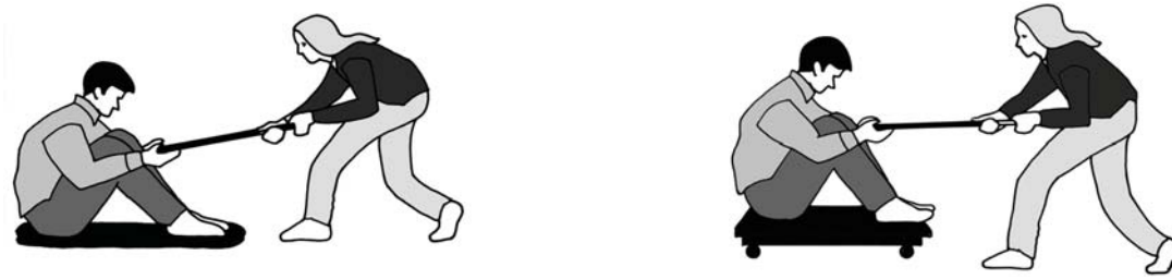
Fig. 5.2. Being pulled with a constant force under two circumstances—(a) sliding along a level floor (while sitting on a relatively smooth floor or on a plastic garbage bag) and (b) rolling along a level floor on a low-friction cart.
