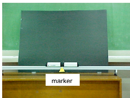
Fig. 3. Two carts of equal masses are initially at rest on the track.
