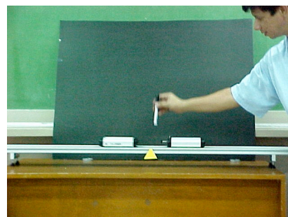
Fig. 4. The plunger is released and the carts move in opposite directions with approximately equal speeds. Note distances covered relative to the marker.
