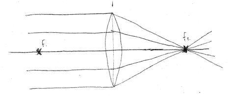
3) Any vay through the center of the lens emerges with unchanged direction
