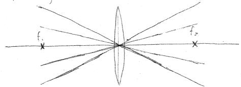
4) All rays that come from a point at the front foral plane emerge from the lens parallel to the ray that crosses through the center
