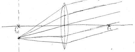
the lens is focused at the back form plane at the point determined by the vay through the center
