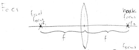
I) Any vay through the front foral point emerges from the lens parallel to the axis
