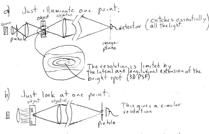
Both a) (b) can resolve points laterally and longitudinally. For b):
