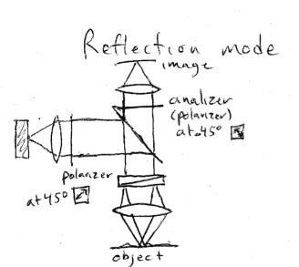
can replace the Wollaston prism with a Nomarski prism po
