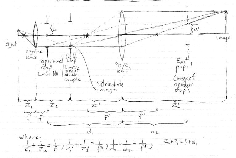
Magnification between object and intermediate image  $M_{\tau} = -\frac{Z_2}{Z_1}$ Magnification between intermediate and final image  $M_{\tau} = -\frac{Z_2}{Z_1}$
