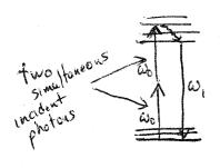
$\omega_i$  is a bit less than  $2\omega_0$ , so  $\lambda_i$  is a bit more than  $\frac{\lambda_0}{2}$ . The two incident photons must be nearly simultaneous, so the probability of emission (and therefore the intensity  $I_i$ ) is proportional to the square of the incident intensity:  $I_i \propto I_0^2$
