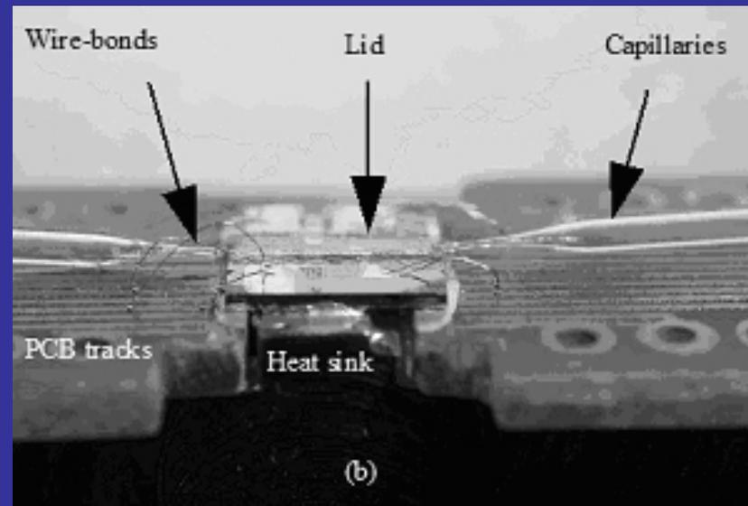
**Photographs of device: (a) mounted on PCB, with tubes leading to pump; (b) fine capillaries feed fluid beneath the glass lid, sealed with NOA-71, and electrical power is provided via wire-bonds from the circuit board**
