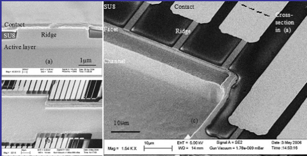
**SEM images of lasers: (a) cross-section through a laser; (b) lasers facing one another across the channel; (c) close-up of facets and channel wall. Note that the channel insulation has not yet been added.**
