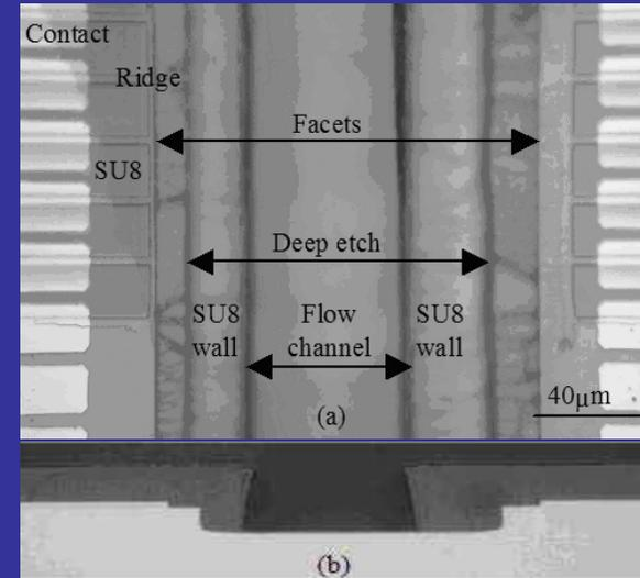
**Photographs of channel with insulation: (a) plan view; (b) cross-sectional view**
