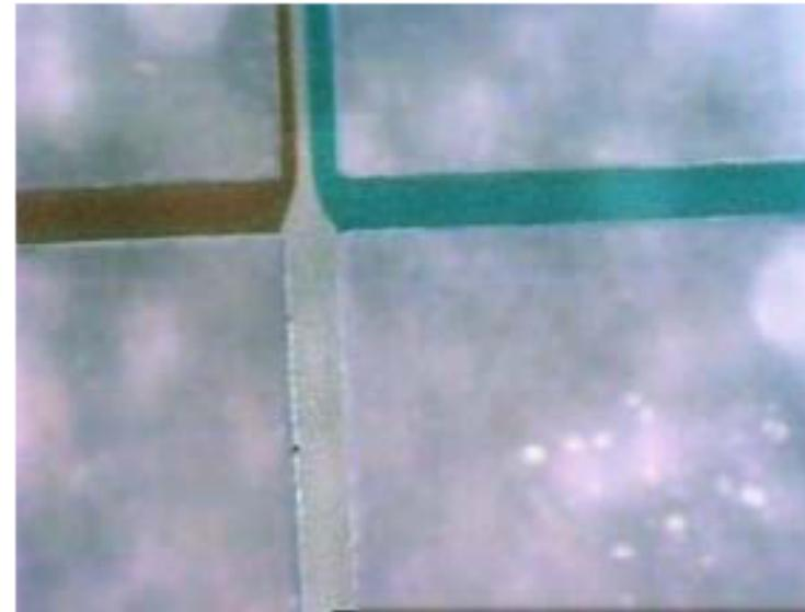
“Characteristic lengths” of microfluidics is 10-100 microns. Typical  $Re < 1$ .
