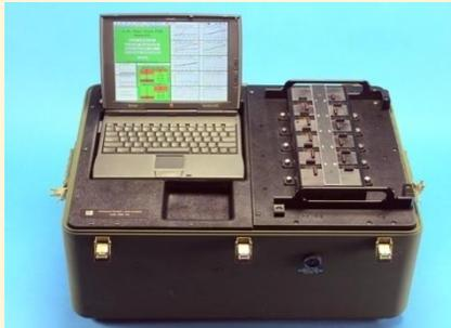
Early prototype , Real-time PCR device
