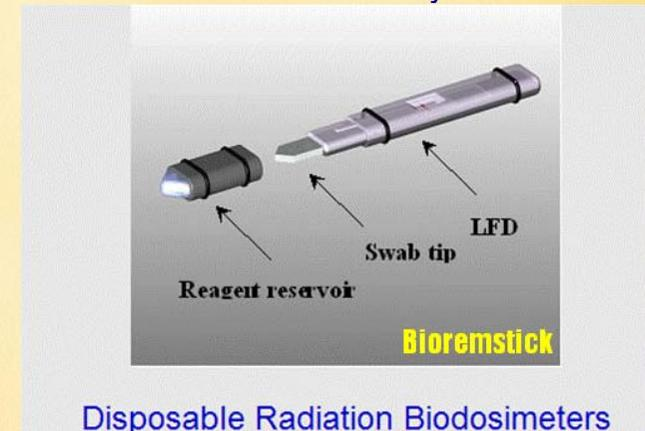
Disposable Radiation Biodosimeters
