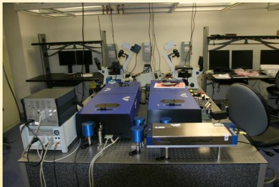
Ratiometric CARS (Coherent Anti-Stokes Raman Spectroscopy) Imaging System
