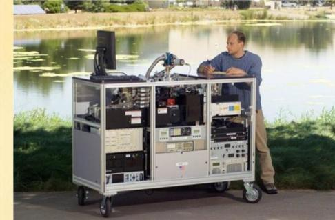
Laser bioaerosol mass spectrometry
