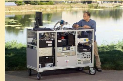
Laser bioaerosol mass spectrometry
