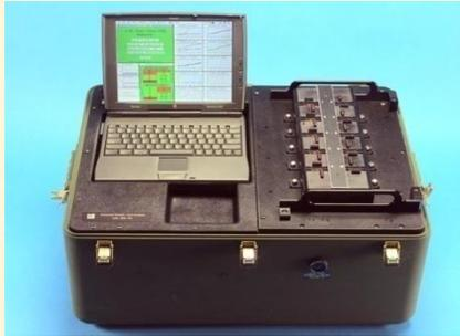
Early prototype , Real-time PCR device
