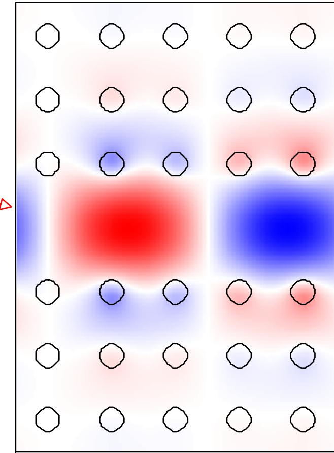
any state in the gap cannot couple to bulk crystal  $\rightarrow$  localized
