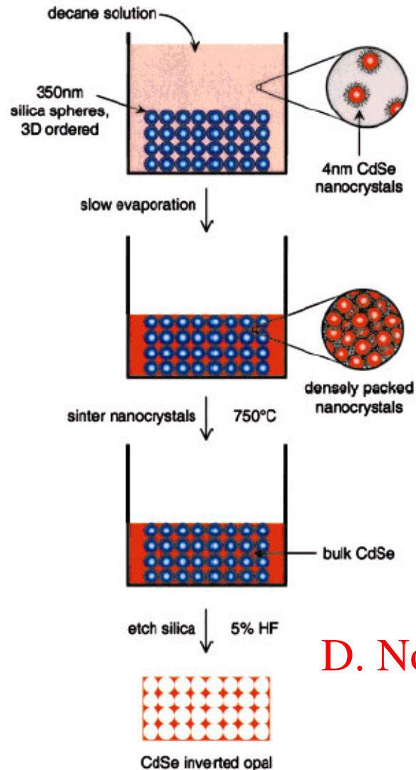
1. Silica PBG immersed in solution of CdSe nanoparticles
