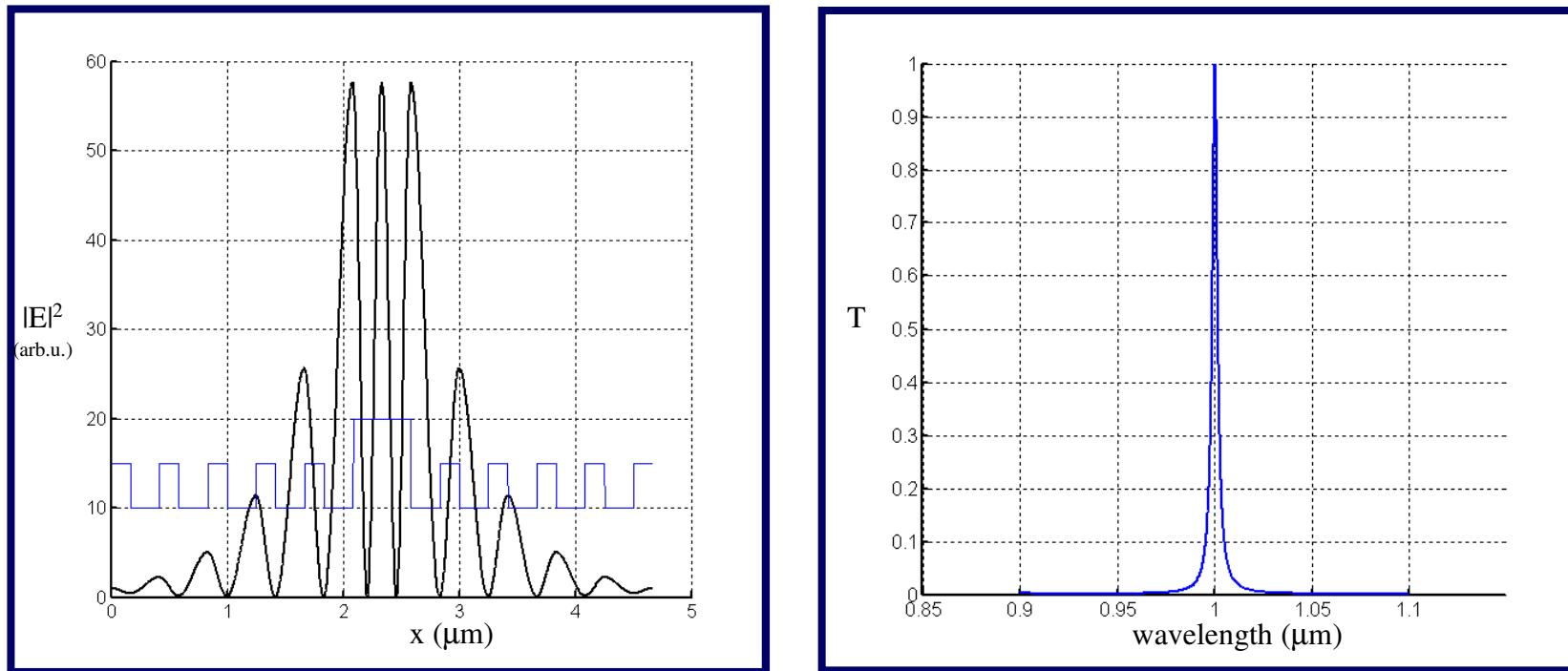
$$Q = 2\pi \frac{\text{Stored Energy}}{\text{Energy lost per cycle}} = \omega_0 \frac{\langle \text{Energy} \rangle}{\langle \text{Power loss} \rangle} \approx \frac{\omega_0}{\Delta\omega_0}$$
