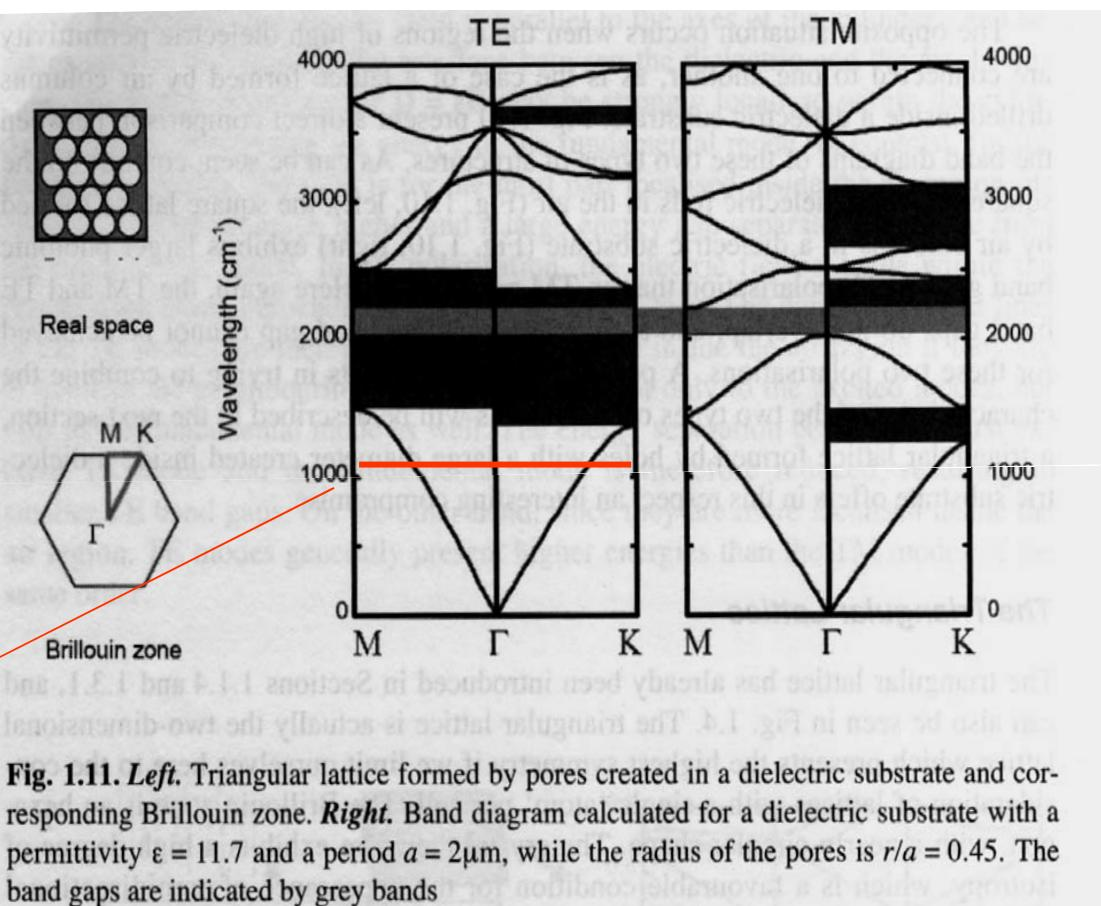
**Fig. 1.11.** *Left.* Triangular lattice formed by pores created in a dielectric substrate and corresponding Brillouin zone. *Right.* Band diagram calculated for a dielectric substrate with a permittivity  $\epsilon = 11.7$  and a period  $a = 2\mu\text{m}$ , while the radius of the pores is  $r/a = 0.45$ . The band gaps are indicated by grey bands
