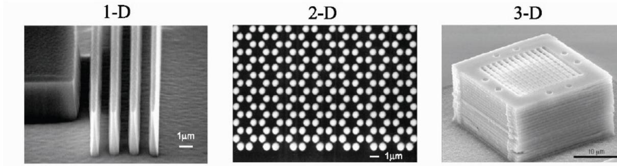
Multi-dimensional periodic structures with a period of the order of optical wavelength.
