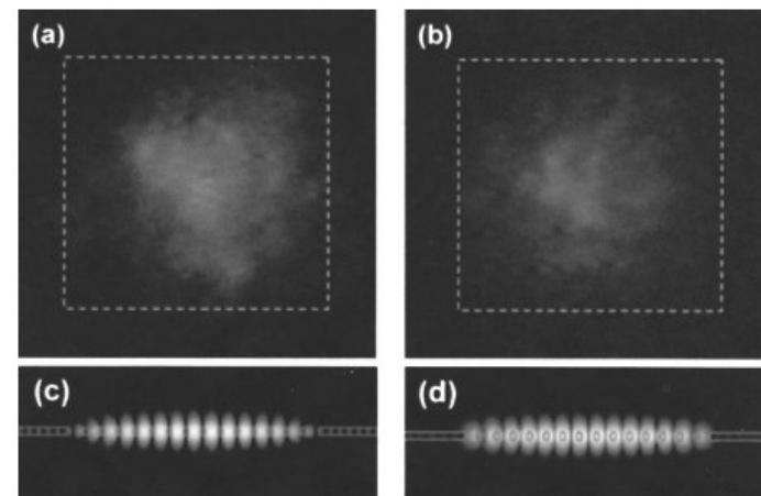
FIG. 2. Mode pattern images of (a) the second X and (b) the second M points bandedge lasers taken by a CCD camera. The dotted squares represent the boundary of the photonic crystal lasers. The side views of the intensity profiles of (c) the second X and (d) the second M points bandedge modes.
