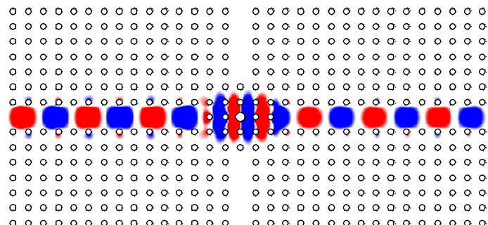
Waveguide crossings ( waveguide + cavity)
