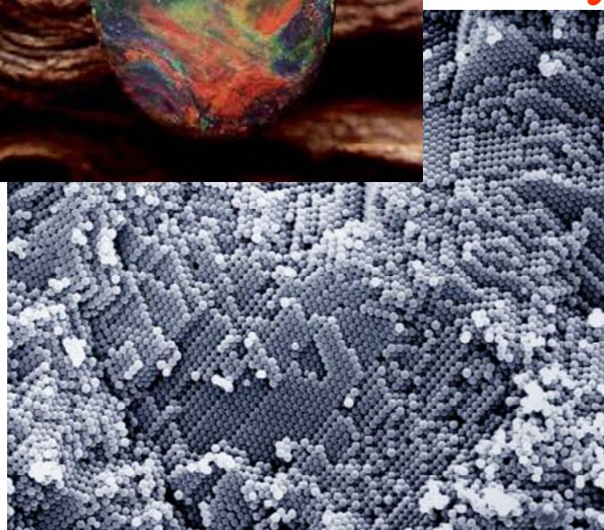
Close packed spheres form a FCC lattice. 3D photonic crystals.
