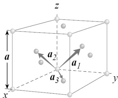
Primitive basis vectors for the face-centered cubic lattice.
