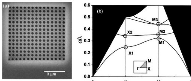
FIG. 1. (a) Top-view scanning electron microscope image of a fabricated square-lattice photonic crystal free-standing slab. The lattice constant and air-hole radius are 550 nm and 210 nm, respectively. Thickness of the slab is 200 nm. (b) The corresponding band structure calculated by the PWE method.
