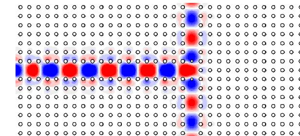
Channel drop filters ( waveguide +cavity)
