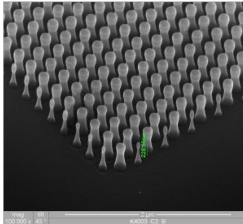
Darren Bagnall at the Southampton University nanofab facility has patterned silicon after the structure of a night flying moth cornea. The moth cornea allows very little light to escape making it an excellent anti-reflective coating.
