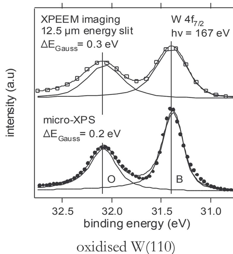
The spectroscopic ability of SPEEM is superior to that of PEEM, because the SPEEM can exploit the full potential of multi-channel hemispherical energy analyzers developed for laterally averaged x-ray photoelectron spectroscopy.
