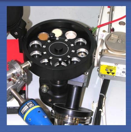
Left: heavy-duty, fully software controlled EDXRF spectrometer (Pd-anode X-ray tube) utilizing 5 secondary targets (Pd, HOPG, Co, Mo, Al<sub>2</sub>O<sub>3</sub>); right: in-house assembled EDXRF spectrometer (Cr-, Fe-, Cu-, Mo-, Rh-, Ag-, W-anode), manual selection of secondary targets (Mo, Rh, Ti in use, any other solid target possible)
