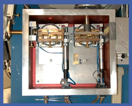
TXRF spectrometers, left: with 12-position sample changer; right: with motorized beam modifier and sample reflector stages
