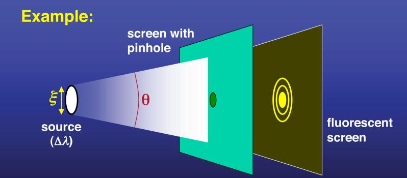
The diffraction pattern may or may not be visible on the fluorescent screen depending on the source size  $\xi$ , on its angular divergence  $\theta$  and on its wavelength bandwidth  $\Delta\lambda$
