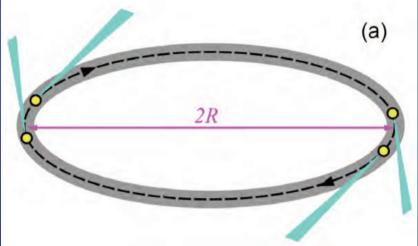
The electrons going around at a speed  $\approx c$  in a storage ring emit synchrotron light like a "flashlight", in a narrow angular cone: why?
