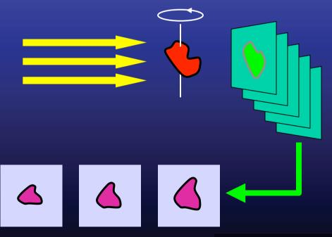
Many x-ray images taken at different angles can be computerreconstructed in three dimensions -- and can even give movies
