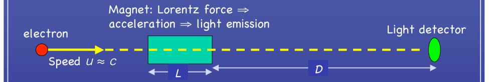
Light pulse starts at (L+D)/c, ends at D/c + L/u, therefore  $\Delta t = L/u - L/c = (L/u)(1-u/c) = (L/u(1+u/c)](1-u^2/c^2)$ For  $u \approx c$ ,  $u(1+u/c) \approx 2c$  and  $\Delta t \approx (L/2c)(1-u^2/c^2) = L/(2c\gamma^2)$ Characteristic frequency  $v = 1/\Delta t \approx 2c\gamma^2/L \Rightarrow$  wavelength  $= c/v \approx L/(2\gamma^2)$ For L = 0.1 m and  $\gamma = 4000$ , the wavelength is  $\approx 30$  angstroms: x-rays!
