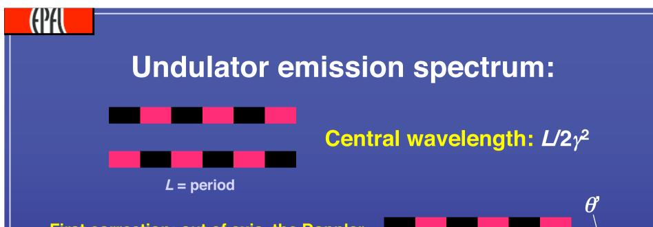
First correction: out of axis, the Doppler factor is not  $2\gamma^2$  but changes with  $\theta^2$ Central wavelength:  $(L/2\gamma^2)/(1+2\gamma^2\theta^2)$
