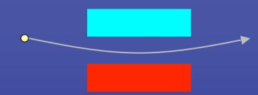
The (relativistic) rotation frequency of the electron determines the (Dopplershifted) central wavelength:  $\lambda_{o} = (1/2\gamma^{2})(2\pi cm_{o}/e)(1/B)$
