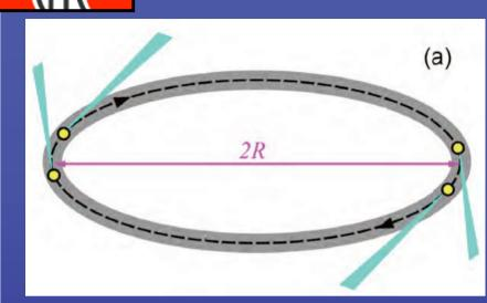
Seen from the side, each electron looks like an oscillating charhe in an antenna, emitting electromagnetic waves with a characteristic frequency  $2\pi R/c$  -- in the radio wave range.
