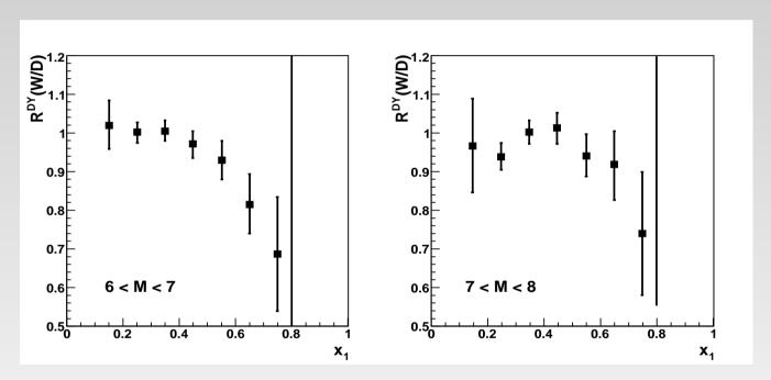
Ratio of DY cross section on W and D as a function of  $x_1$ , at large dilepton masses to eliminate nuclear shadowing
