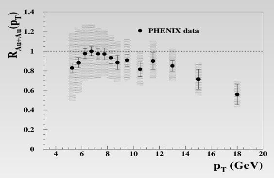
Nuclear modification factor for direct photon production in  $\boldsymbol{Au+Au}$  collisions as a function of  $\boldsymbol{p_T}$
