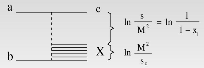
— the probability to radiate no gluons in the rapidity interval  $\Delta y = ln \frac{1}{1-x_1}$  is suppressed by the SUDAKOV'S FORM FACTOR  $S(\Delta y)$ , which violates QCD factorization
