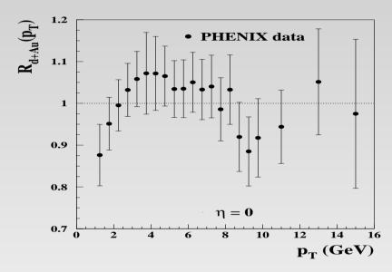
Nuclear modification factor for large- $p_T$  neutral pion production in d + Au collisions as a function of  $p_T$
