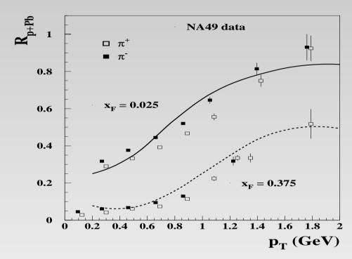
Nuclear modification factor for pions in p + Pb collisions as a function of  $p_T$  for two different fixed values of  $x_F$
