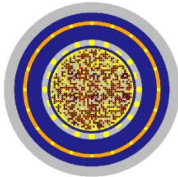
FIG. 4.43. Core modeling in Monte-Carlo code TRIPOLI4 (“Improved PB modeling”).
