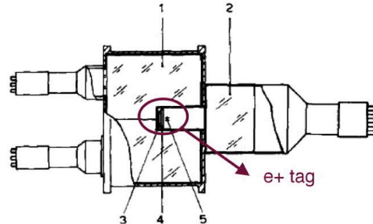
Fig. 1. Schematic view of the set-up: (1): NaI calorimeter; (2): NaI counter (3): target; (4): proportional counter; (5): the positron source  $^{22}\text{Na}$ .
