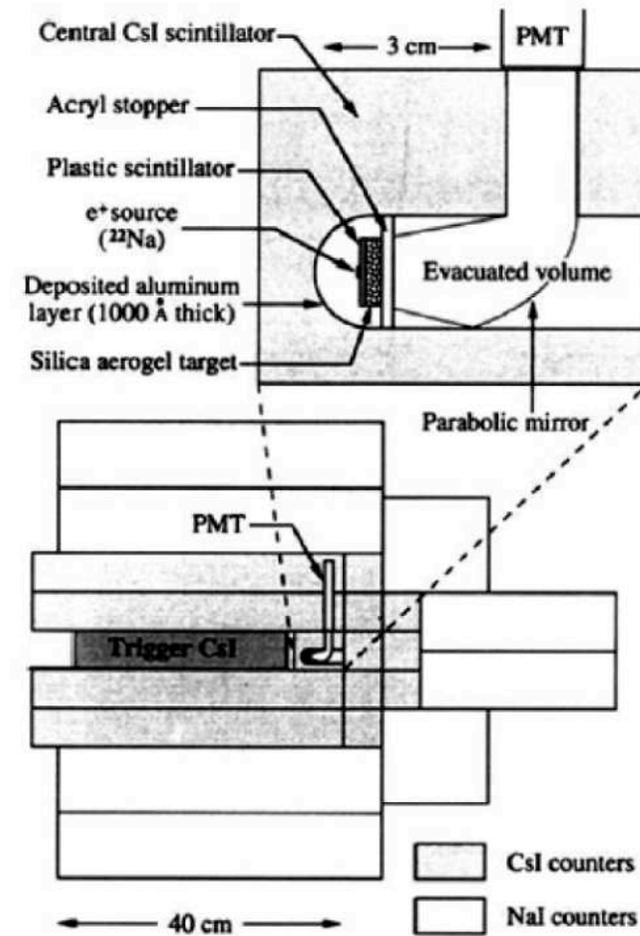
FIG. 1. Schematic of the experimental setup.
