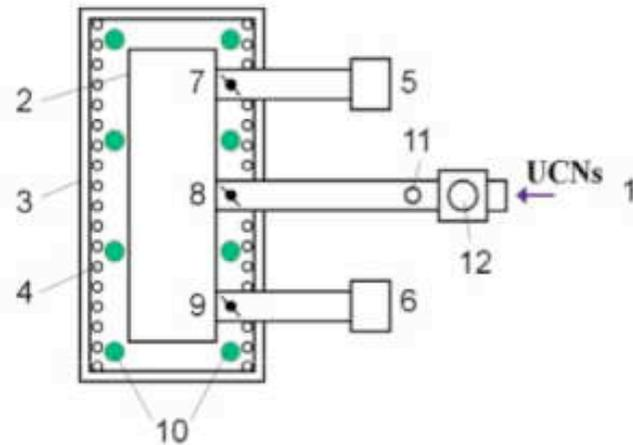
1: UCN input guide; 2: UCN storage chamber; 3: magnetic shielding; 4: solenoid; 5-6: UCN detectors; 7-9: valves; 10: Cs-magnetometers, 11: monitor detector, 12: entrance valve.
