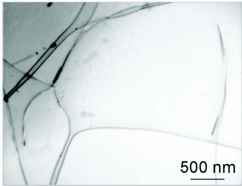
Transmission electron microscopy of plastically deformed GaAs (diffraction contrast image)
