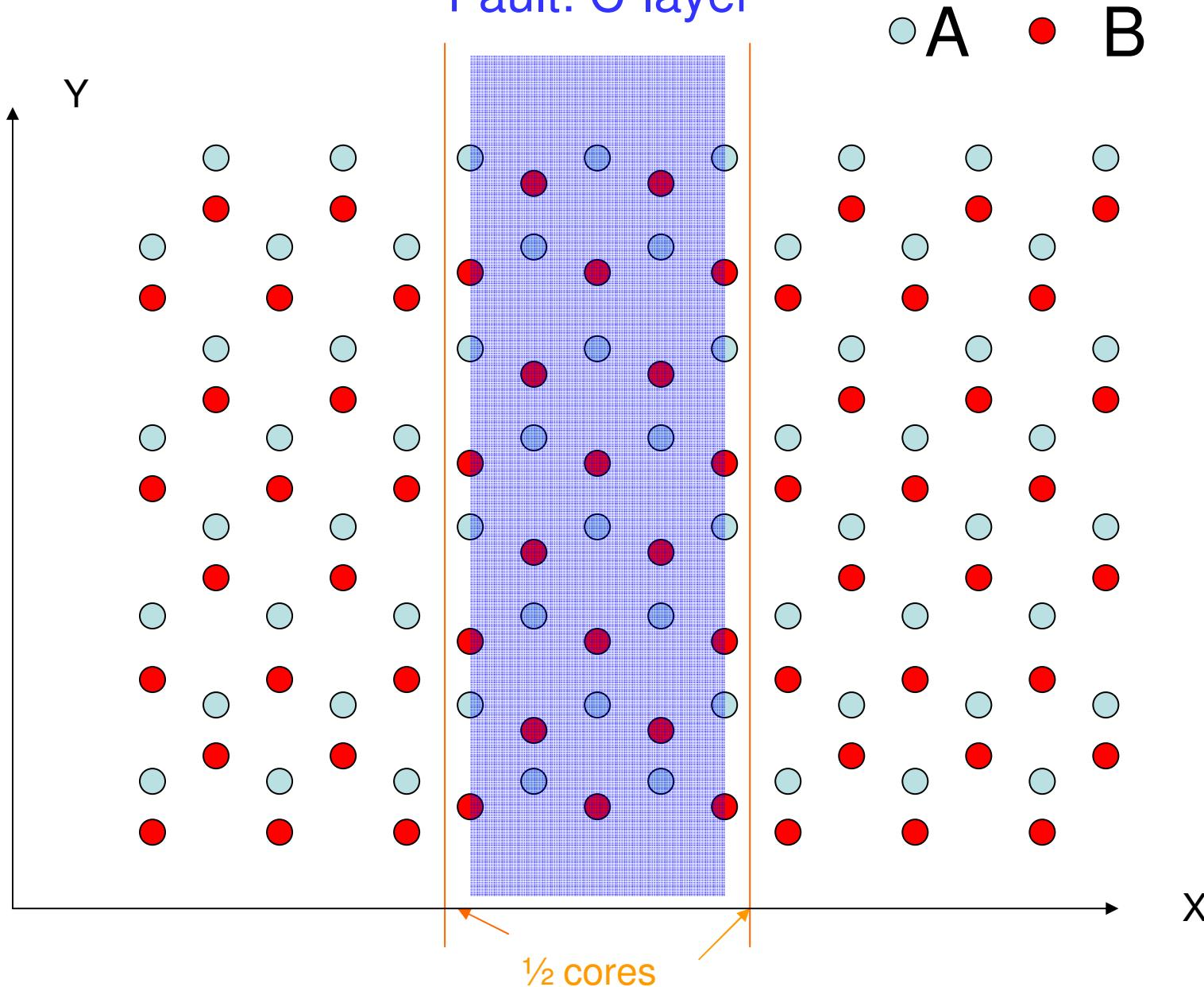
Columnar view of fault + split core: many layers
