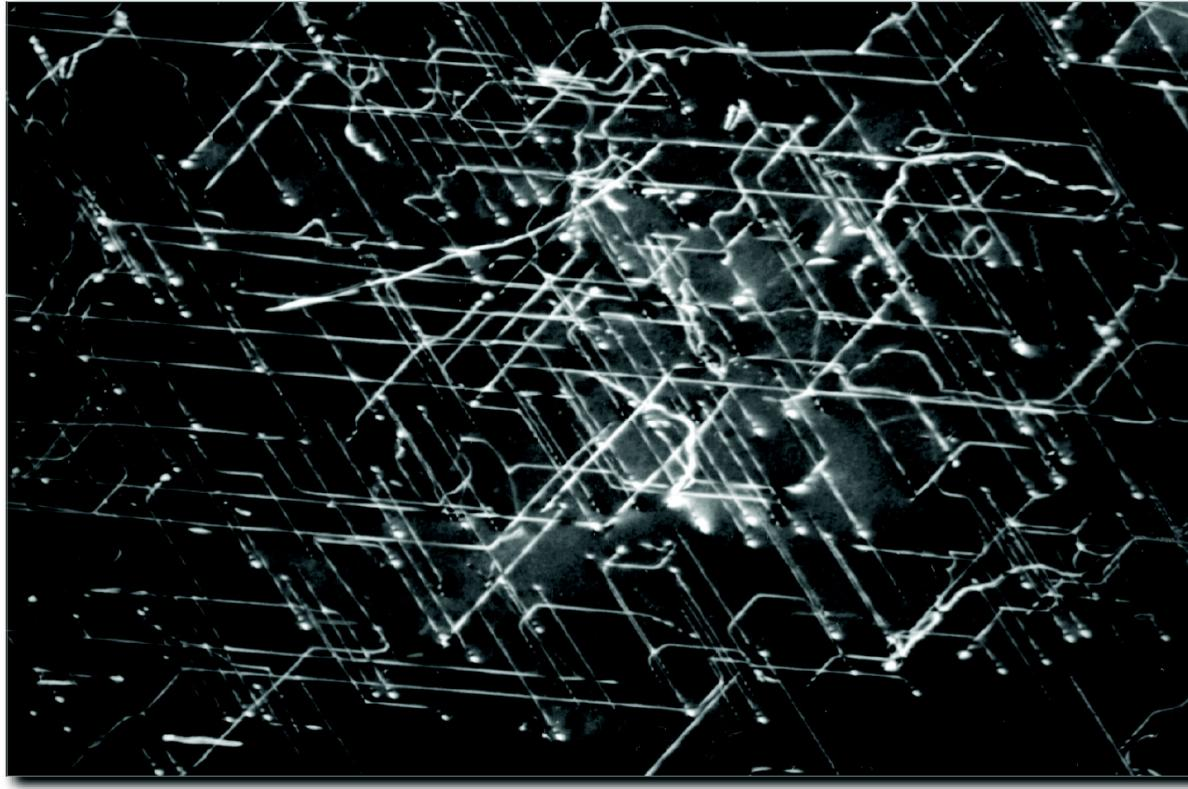
TEM image of dislocations in silicon plastically deformed in a single-slip
