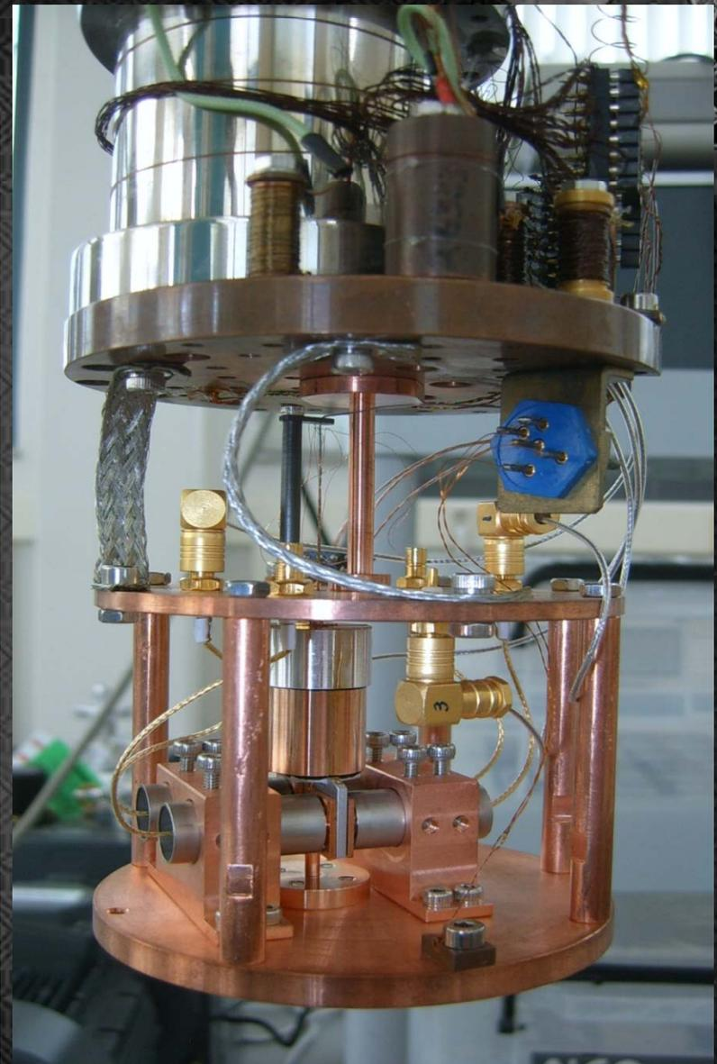
Resonant frequency 738 Hz, Q-factor  $8 * 10^5$
