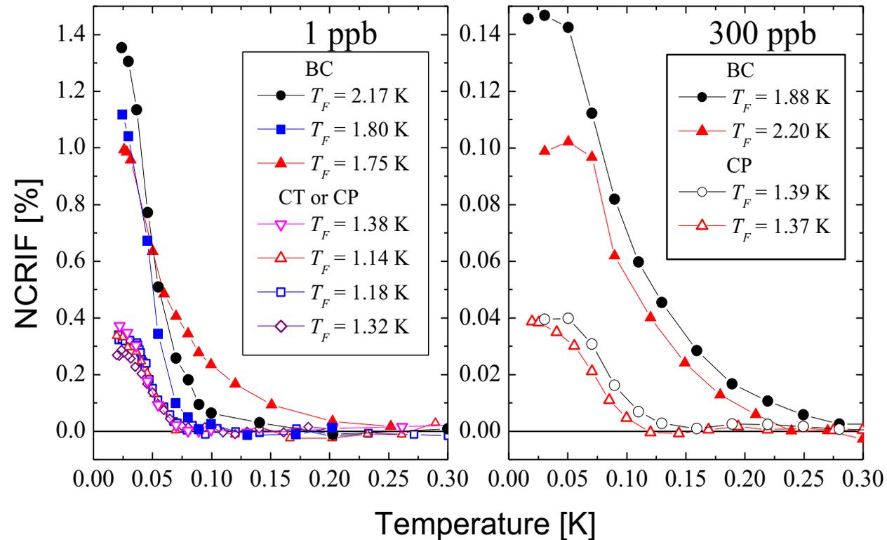
Comparing BC samples to CP/CT samples for two different sample cells. Note the factor of 10 difference in NCRIF.
