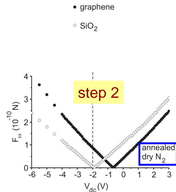
graphene annealed at 150 deg C for 1 hour in flowing N<sub>2</sub>
