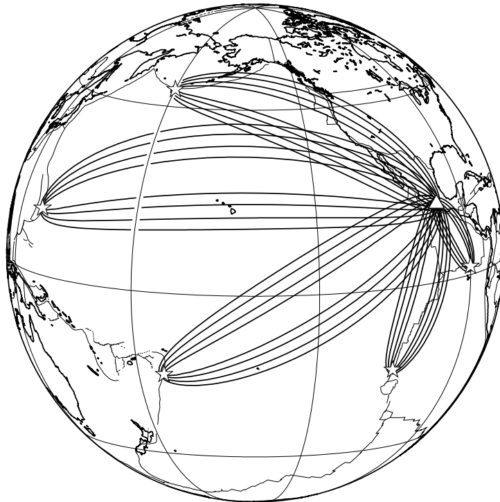
Figure 4: Rayleigh wave sensitivity-zones ( N = 8/3 ) for waves observed in Mexico (triangle) originating from several epicentral regions (stars): Galapagos (2087 km), East Pacific Rise (4493 km), Aleutians (7777 km), Tonga (8916 km), and the Marianas (11700 km). These sensitivity-zones are for 20 s, 50 s, 100 s, and 150 s Rayleigh waves, where the zone is narrowest at shortest period.
