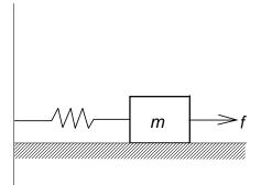
Let x be a deviation of the mass from the equilibrium. The force f is friction opposing the motion of the mass. Denote K a measure of the spring's stiffness.
