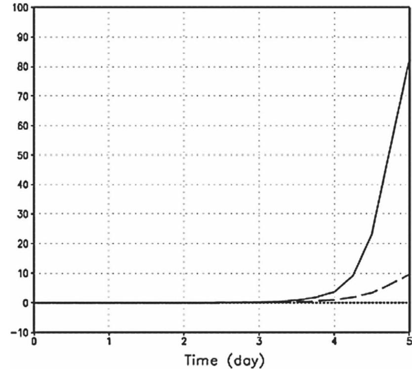
**Right:** Evolution of maximum perturbation kinetic energy under a constant easterly shear (solid line), westerly shear (dashed line), and zero shear (dotted line). JJA SST and surface moisture fields are specified.
