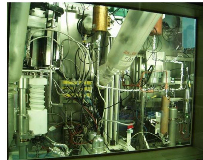
On-line gamma spectrometers (ex. on the fuel ↓)
