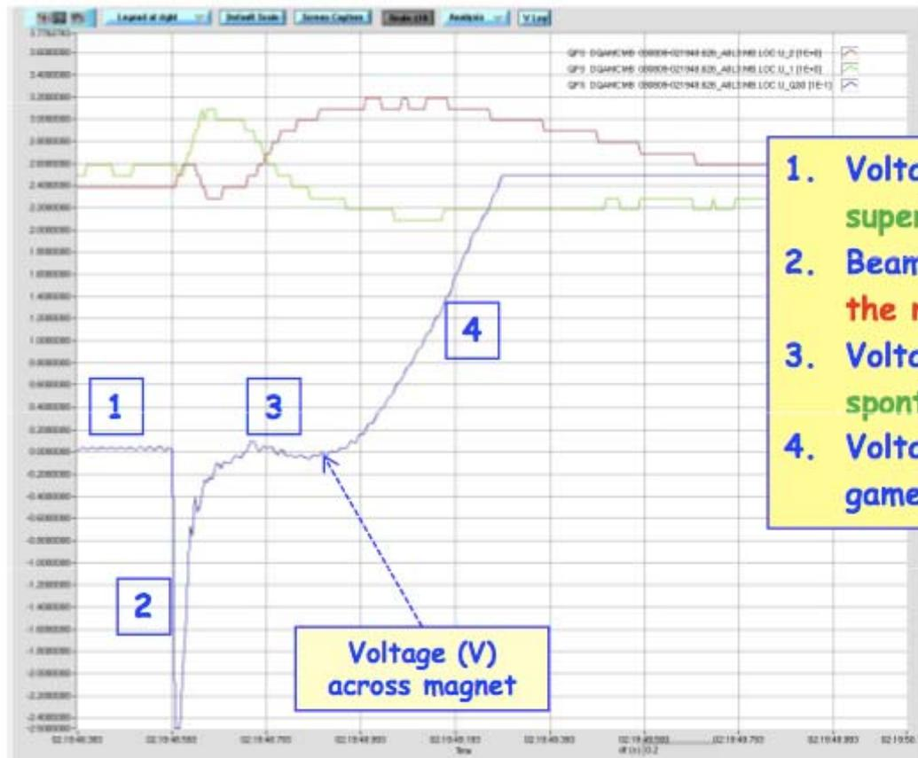
1. Voltage = 0, no resistance, magnet is superconducting.
