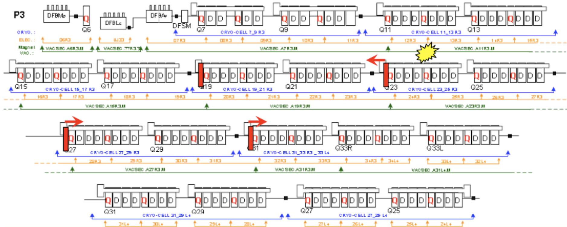
**Insulating vacuum barrier every 2 cells in the arc → Some moved**
