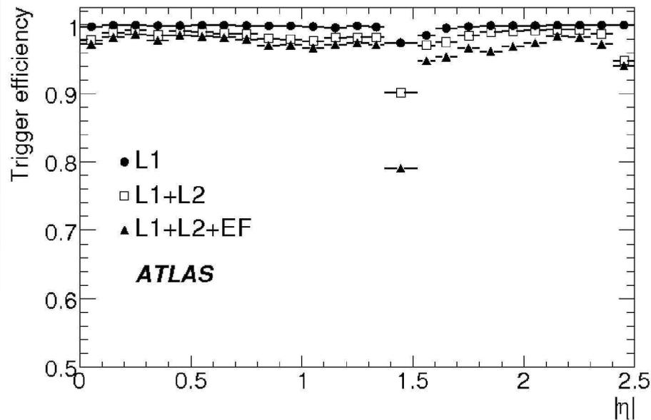
Efficiencies for single electrons ideal geometry sample with  $7 < E_T < 80$  GeV for the e10 trigger as a function of  $\eta$ .
