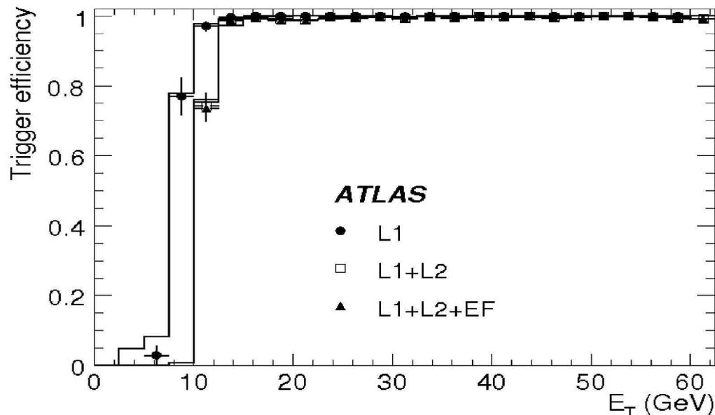
Tag and probe for 2e10 trigger.
