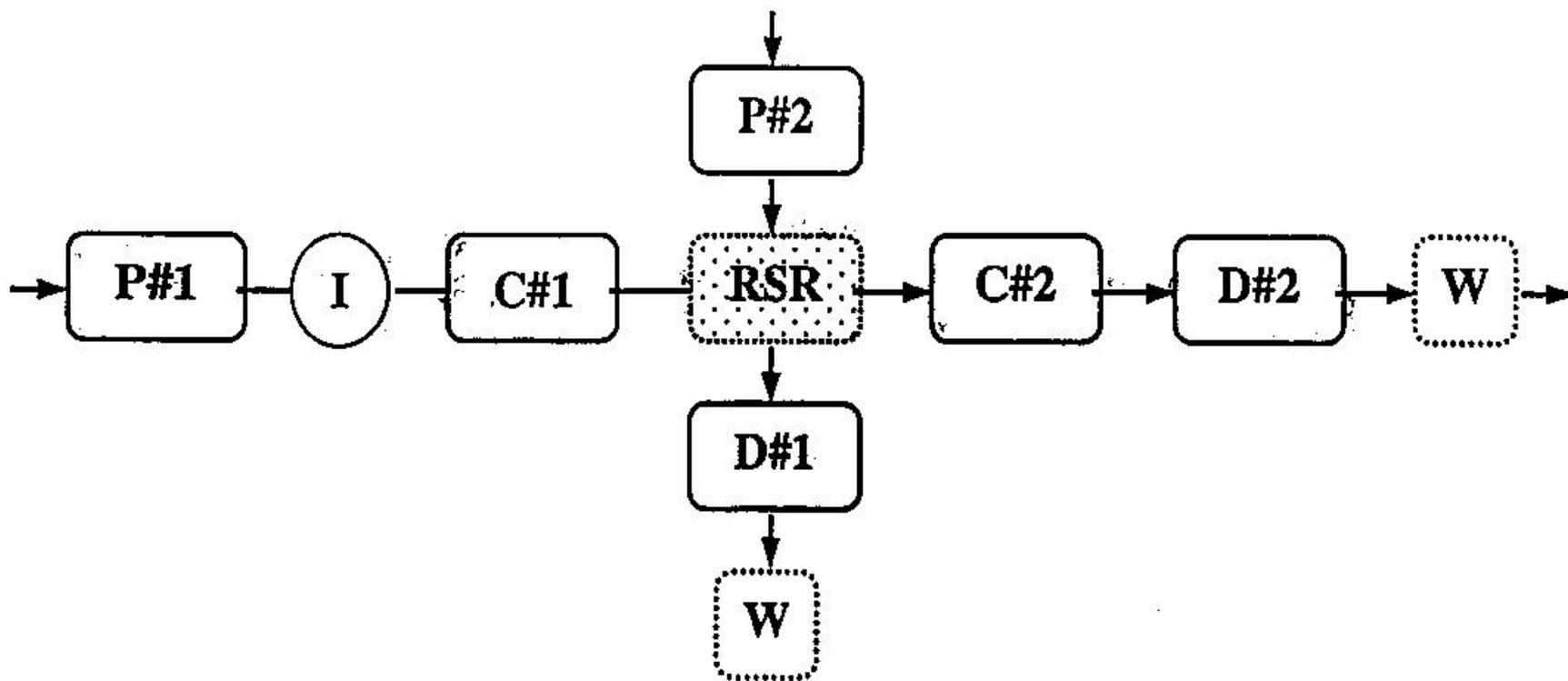
*P = pump; I = injector; C = column; D = detector or system of detectors; W = waste*
