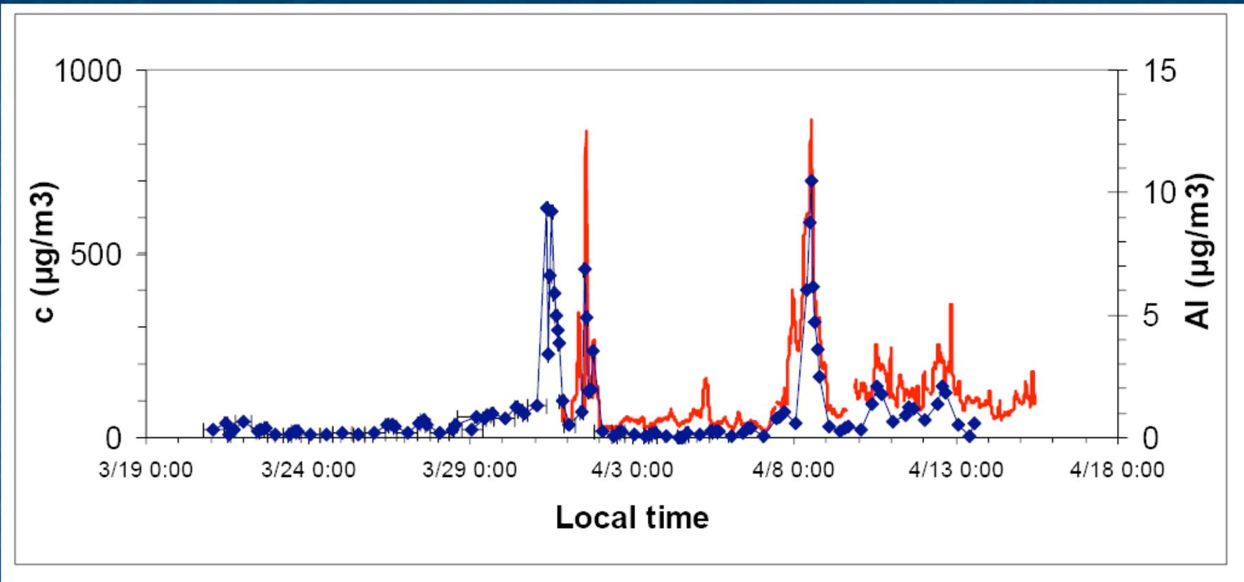
**Figure 1:** Evolution with time of the PM10 mass concentration ( $c$ , solid line) measured in real time by the TEOM microbalance and of the Al mass concentration retrieved by XRF analysis of aerosol samples collected on nuclepore filters (losanges).
