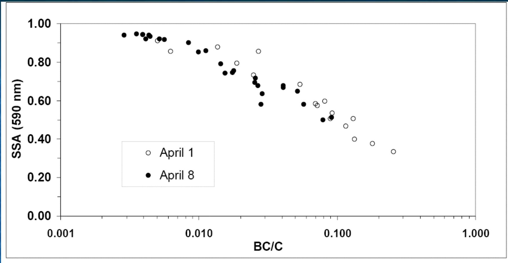
**Figure 10:** Sensitivity of the single scattering albedo at 590 nm to the proportion of the UP/MD mixture. Uncertainties on values corresponding to UP-dominated situations (larger values of BC/c) are ca. 15% whereas uncertainties corresponding to situations with a strong mineral dust component (lowest values of BC/c) are ca. 3%.
