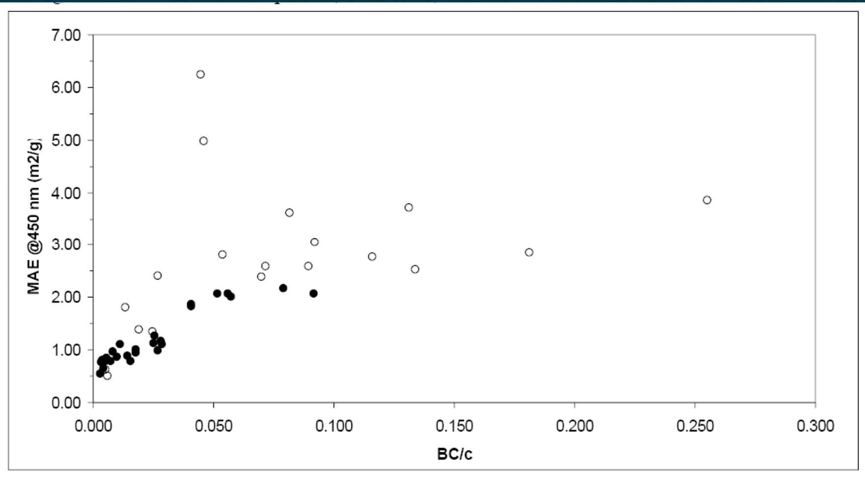
**Figure 5:** Influence of the proportions of the urban pollution/mineral dust mixture on the aerosol mass scattering efficiency at 450 nm. Results for April 1 (open circles) have been distinguished from those of April 8 (full circles).
