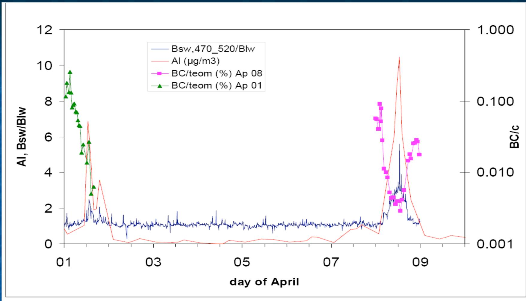
**Figure 9:** Ratio of Angström's exponents for absorption at short wavelengths (BSW computed between 470 and 520 nm) and at long wavelengths (BLW). This ratio is sensitive to the presence of dust in the mixture (indicated by large Al concentration, and negatively correlated to BC/c).
