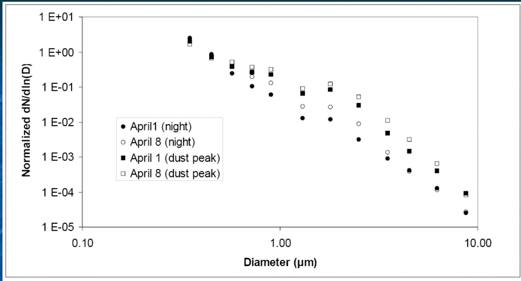
**Figure 4:** Size distribution of the aerosol mixtures measured by the optical size analyzer in situations dominated by urban pollution (April 1 and 8 nights) and at the peaks of the two dust events. In order to facilitate comparison, values have been normalized to the total particle concentration.
