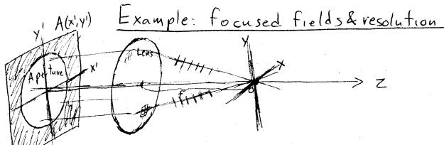
The lens focuses the light though the aperture.
