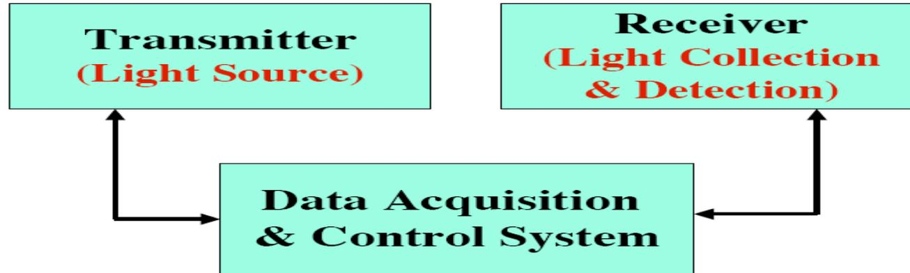
**Transmitter** (laser pulses that meet some requirements): wavelength, frequency accuracy, bandwidth, pulse duration time, pulse energy, repetition rate, divergence angle, etc
