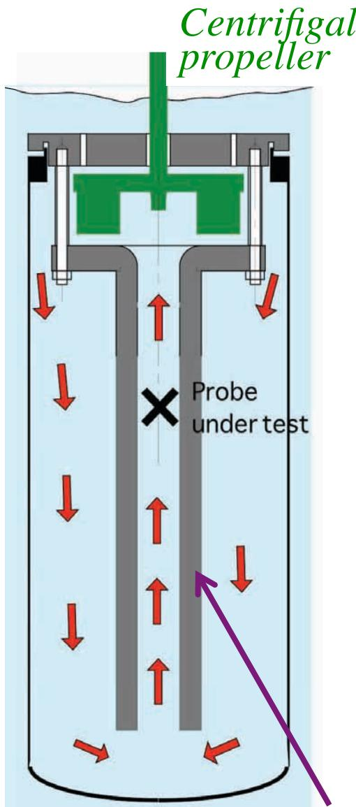
$\Phi = 23 \text{ mm}$ ,  $L \sim 250 \text{ mm}$ ,  $V$  : up to  $1.3 \text{ m/s}$
