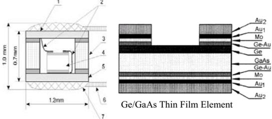
1 and 5: copper discs; 2: gold strip; 3: corundum cylinder; 4: Ge/GaAs sensitive element; 6: copper wire; 7- tin.
