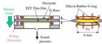
Fig. 3 The bimorph construction of the diagram and its mounting.
