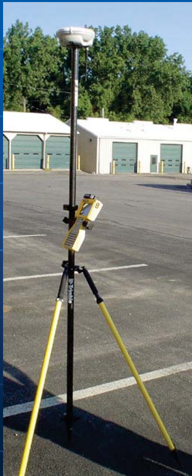
Trimble 5800 Receiver and TSC 2 Controller Rover Assembly Mounted on the Range Pole and Bipod
