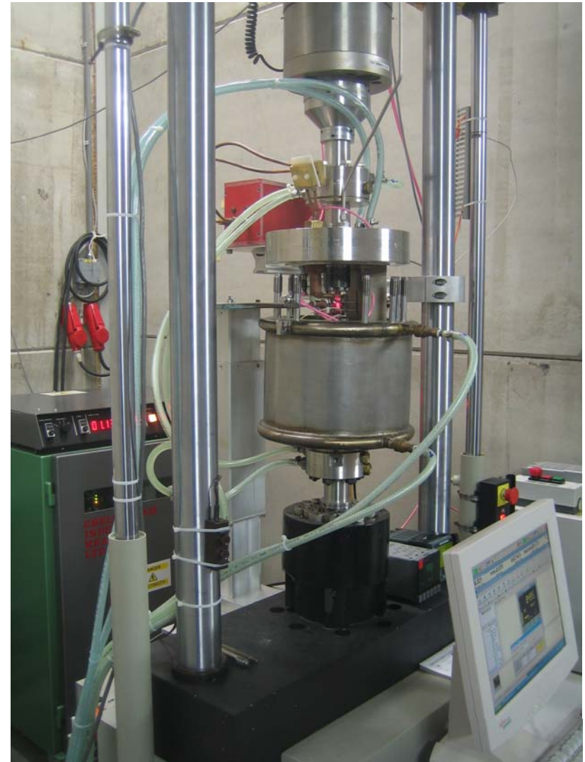
Setups for low pressure (left) and high pressure (right) environmental LCF/TMF tests
