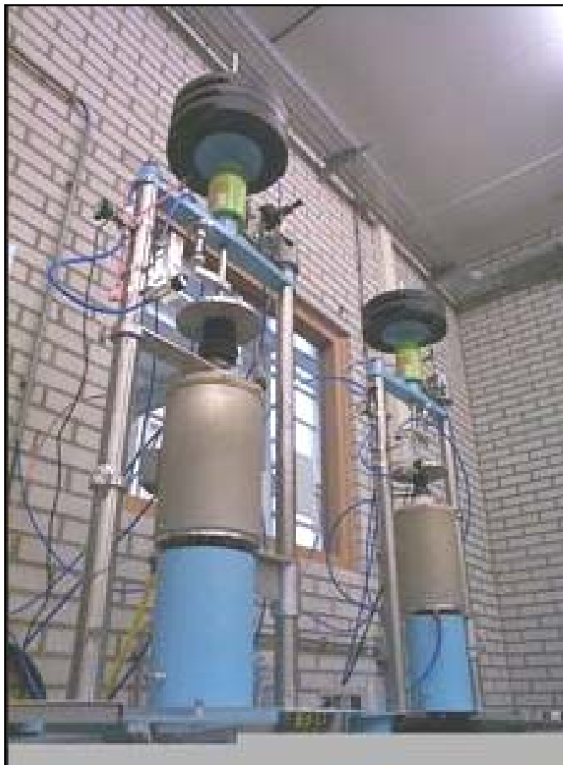
SP creep test rigs at JRC-IE
