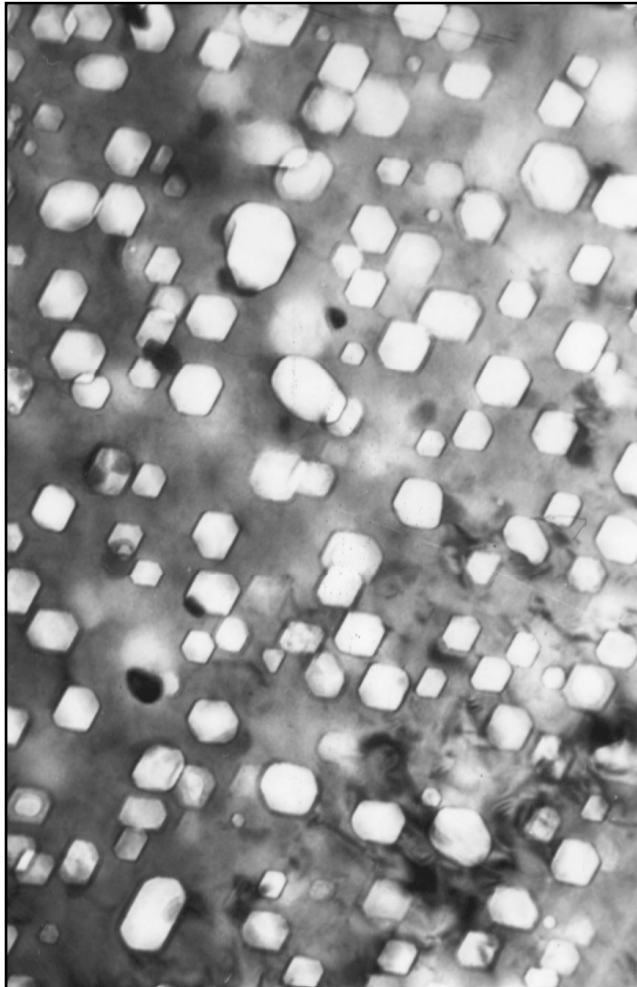
Austenitic SS: ChS-68 CW (ЧС 68 ХД), Very high swelling (many big voids)
