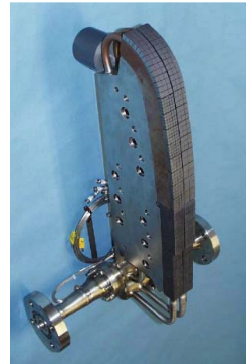
EU Prototype of Inner Vertical Target with CfC & W Armour
