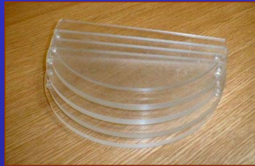
PMMA mammography phantom
