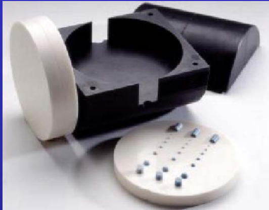
CIRS Helical CT Phantom - Model 061
