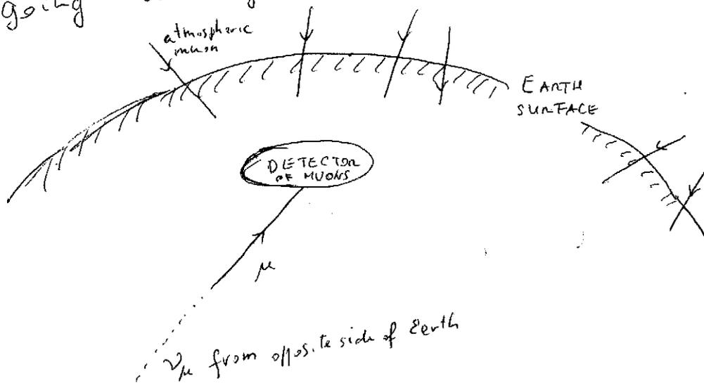
MUONS COMING FROM BELOW CANNOT BE OF COSMIC ORIGIN, MUST BE  $\nu_\mu$  CONVERTED INTO  $\mu^\pm$
