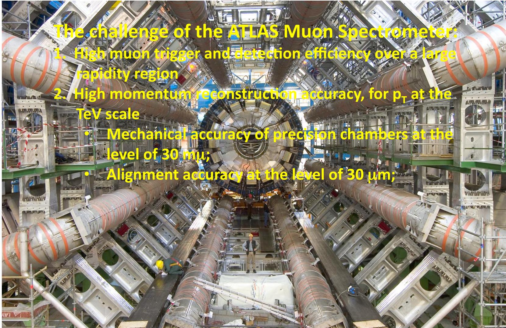
**The challenge of the ATLAS Muon Spectrometer:**
