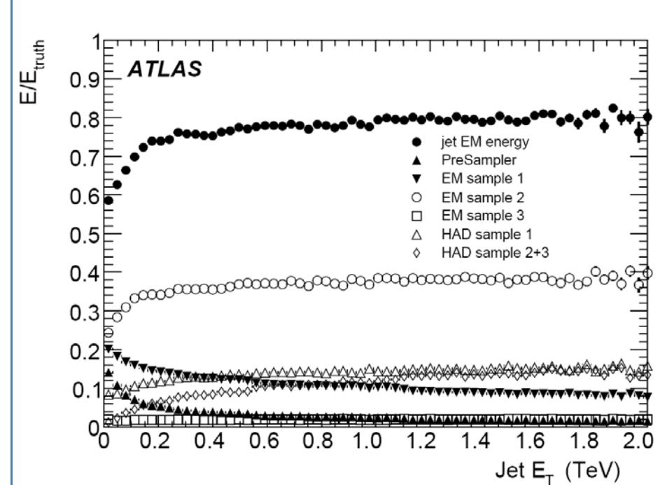
60-80% of true jet energy in LAr EM calorimeter, for  $|\eta| < 0.7$  central region
