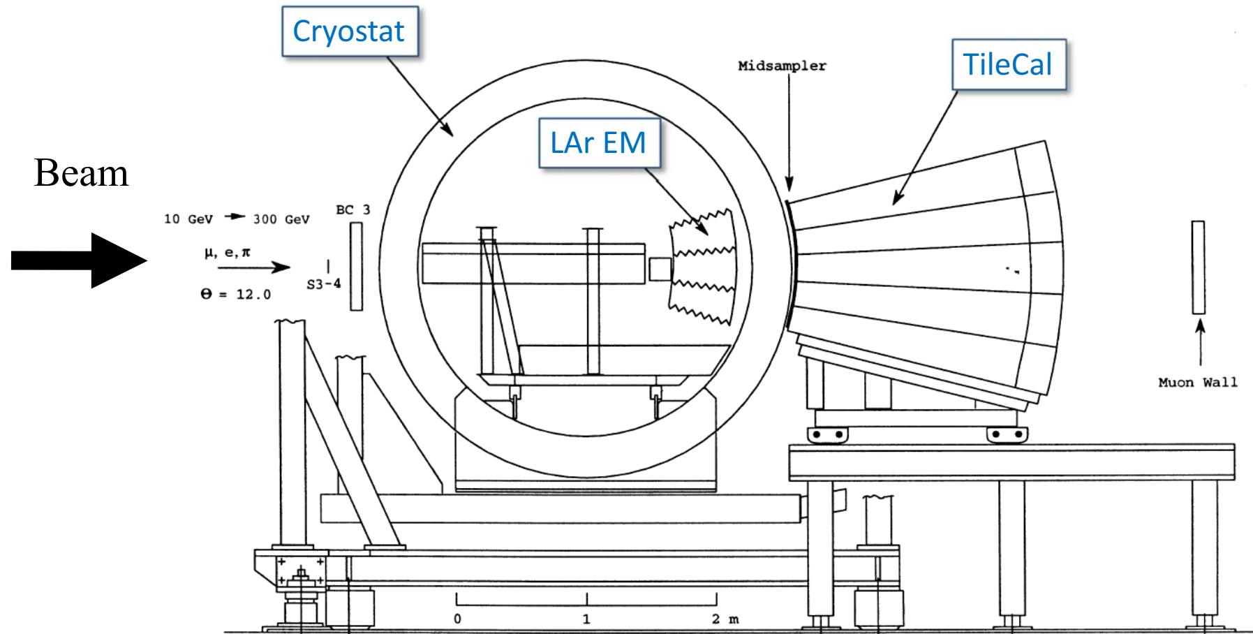
Calibrate with particle beams of known energy up to 300 GeV.
