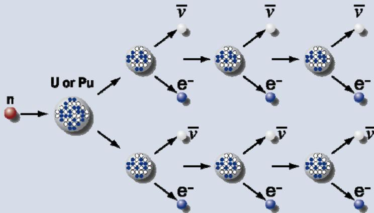
About  $10^{22}$  antineutrinos are emitted per second from a typical PWR unattenuated and in all directions
